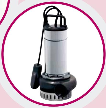
Electric pumps with set back opening impeller or vortex type and with generous free passages are ideal for handling screened water, effluent or for emptying small community septic tanks. Vortex type impeller versions are recommended where the liquid pumped contains solid matter in suspension or fibre. On request M pumps can be supplied complete with an automatic coupling at the discharge for use in effluent or septic tank installations.
