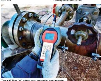
The KATFlow 200 offers easy, portable, non-invasive flow measurement, according to Katronic.
