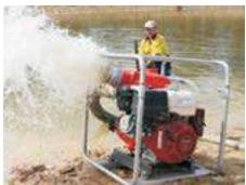
Australian Pump manufacturers 2", 3" and 4" portable pumps that are available in either petrol or diesel drive. The Aussie trash pump range is designed to
