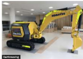
Komatsu Reveals the Concept of the First Fully Electric and Remote-Controlled Mini Excavator
