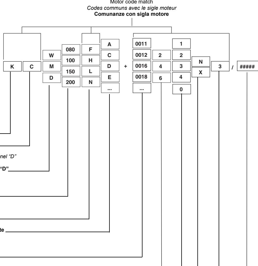
**Standard electric pump: (N) ; explosion-proof version: (X) (construction according to EN60079-0 EN60079-1 standards type ATEX II 2G Exd IIB T4)**
