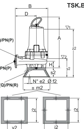
For fixed installation in a dry chamber - vertical (/R)
