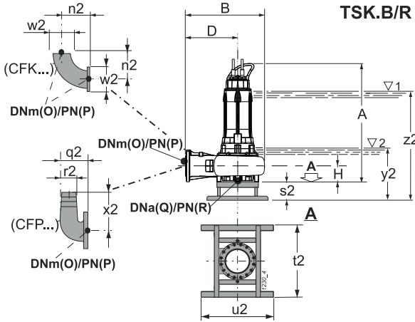
For fixed installation in a dry chamber - vertical (/R)
