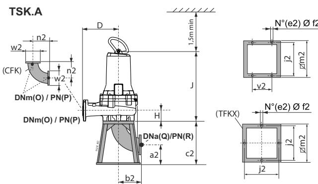
For fixed installation in a dry chamber - horizontal (/R)
