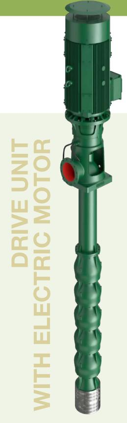
The pump shaft is coupled to the motor shaft by a flexible coupling. The drive unit is fitted with an independent support with thrust bearings to support the rotating assembly. The bearings are angular-contact ball bearings, with grease lubrication for low and medium power drives, while oil-lubricated spherical roller bearings are used for the higher power drives and cooled by an extremely efficient cooling device.
