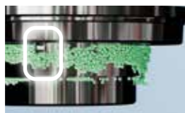
Solid body anti-sedimentation system
