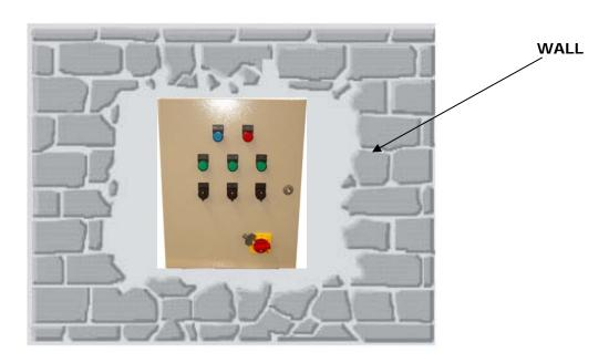
N.B.: DO NOT INSTALL THE ELECTRIC CONTROL PANEL IN THE VICINITY OF OBJECTS WHICH ARE IN CONTACT WITH FLAMMABLE LIQUIDS, WATER OR GAS;
